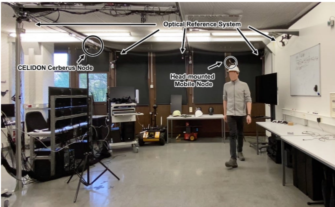
Fig. 7. Annotated picture of the experimental setup. The CELIDON Cerberus node is mounted statically on a pole. A mobile node based on the same hardware, but equipped with a single antenna is mounted to a helmet. Ground-truth is provided by an optical reference system.
